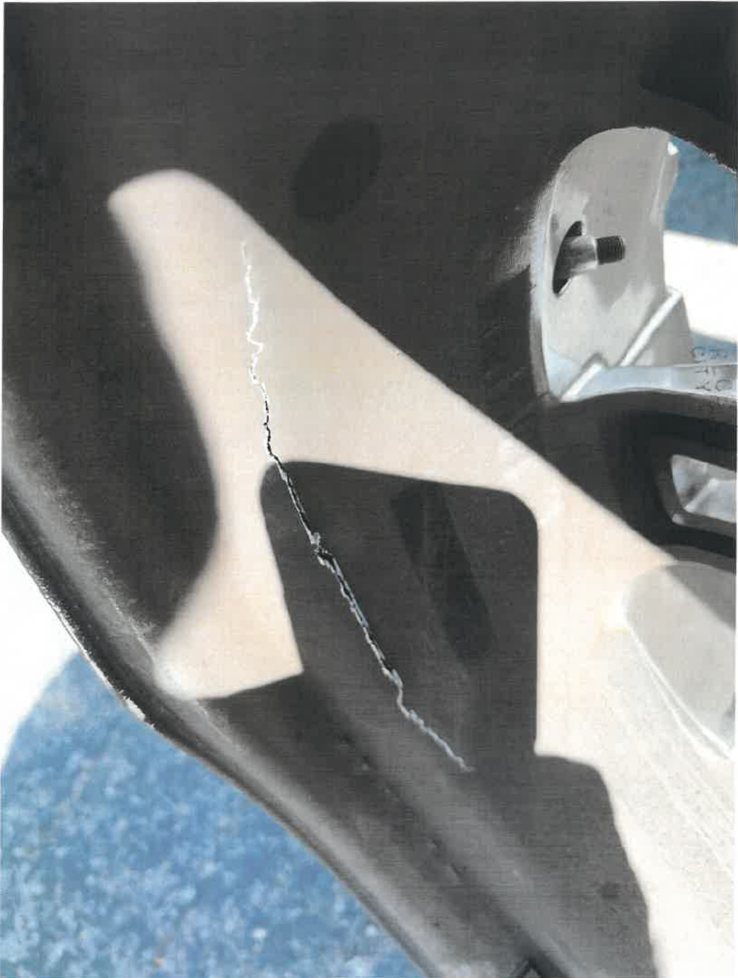
Exhibit C4 – Cracked and Bent Rim
