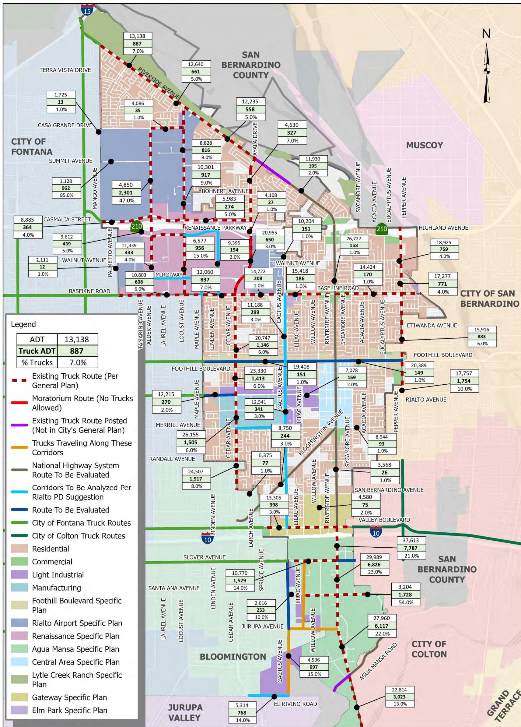
Figure 14 – Existing and Evaluated Truck Routes With ADT, Truck Volumes, and Truck Volume Percentage
