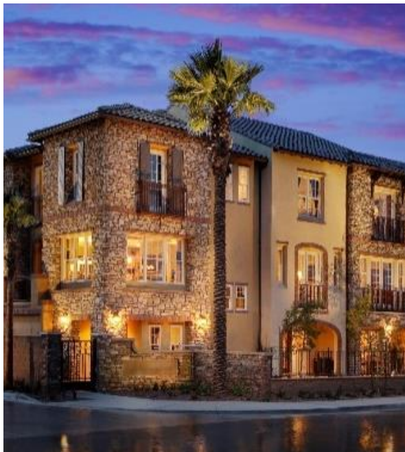
Example, Material Changes at Inside Corners
