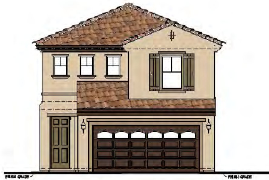
FRONT ELEVATION A - PLAN 2 - SPANISH SCHEME 2 SCALE: 1/8"=1'-0"
